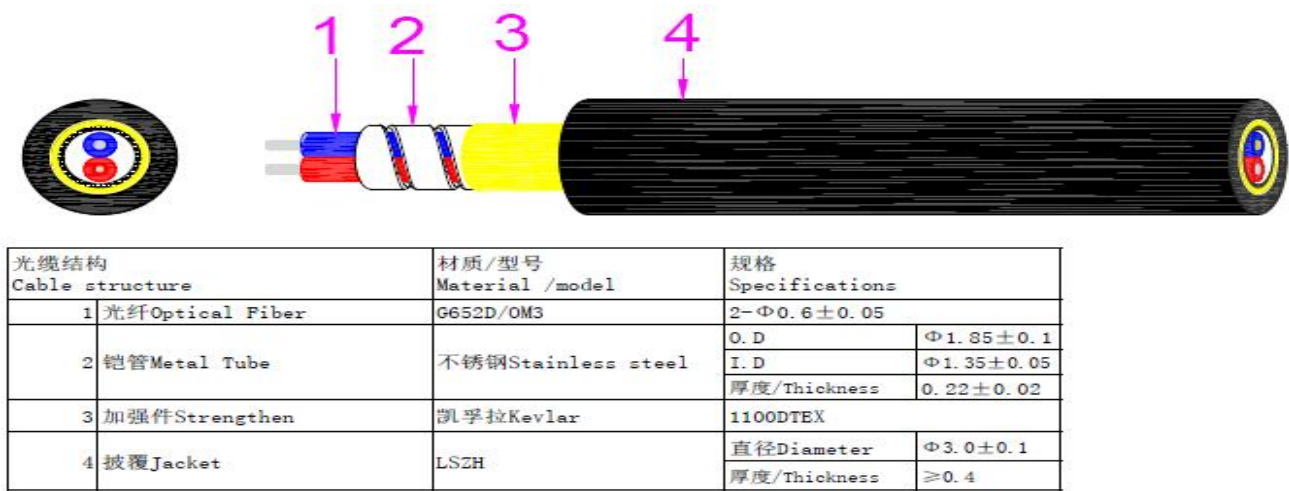
Figure6. Hardened optical cable Specifications
